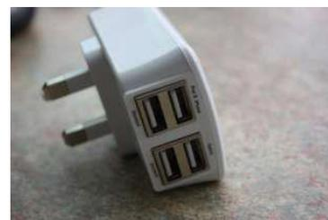
that there was a risk of electric shock. In addition the plug pins were not even made to British Standard sizes or spacing and as a result the poor engagement of the pins with a standard wall socket could lead to arcing and fire, according to the expert report commissioned by Trading Standards.
